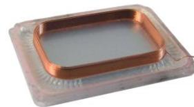
Figure 3: Micro speaker diaphragm with voice coil
