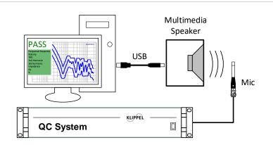
The stimulus is played back with a 3rd party audio device (USB audio device) with unknown delay. The synchronization is performed dynamically through the acoustical measurement channel. Subsequent measurements use the detected delay to trigger the analysis in the quasi-synchronous playback process.
