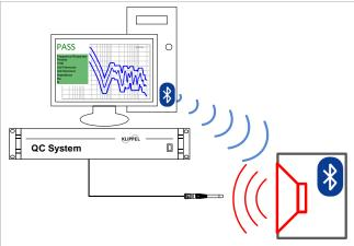
This setup is similar to the USB speaker example above, but the test signals are transferred wirelessly via Bluetooth.
