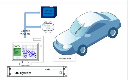
If the device under test (in this example an automobile audio system) does not provide an accessible auxiliary signal input, the stimulus sequence must be transferred offline to the audio system.
