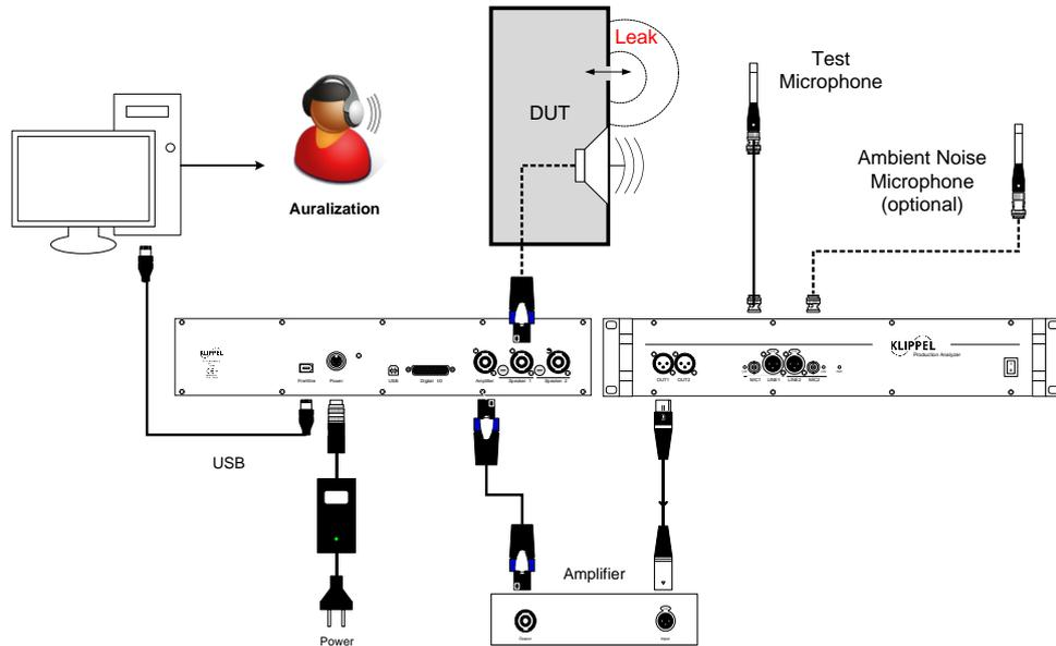
The schematic shown above illustrates the typical hardware setup for passive audio system diagnostics with ALS.
