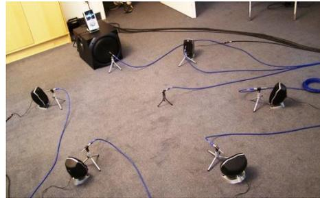
*Testing a 5.1 system under free air conditions*
