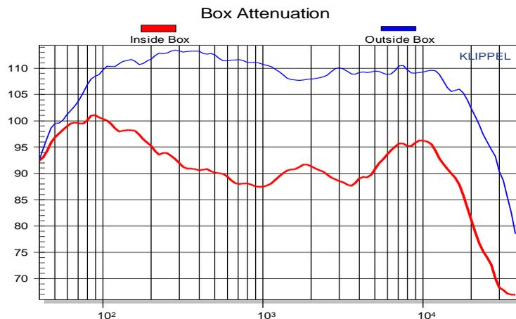
Typical attenuation of a simple test enclosure (red curve: inside box, blue curve: outside)
