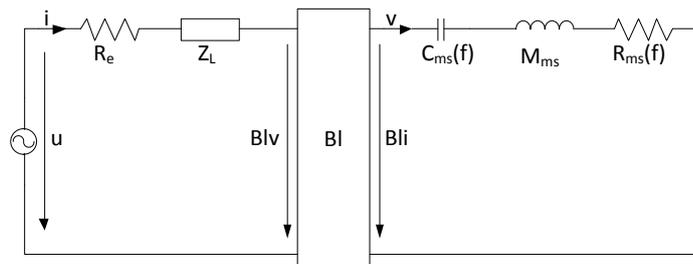
Figure 1 Equivalent electrical circuit used as linear transducer model
