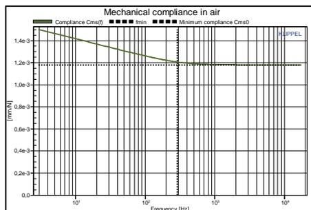
**Result Curve 7 Frequency dependence of mechanical compliance**
